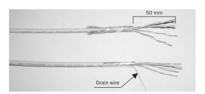
Strip approximately 50mm from the cable jacket, fold back the foil or braid shield, and separate the wire into 4 pair each.
