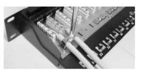
Fasten the screws through metal case to hold tightly down for two cable jackets in the same time.
