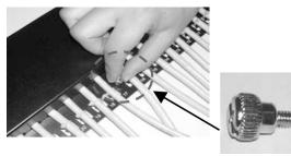
Place the metal cover onto the bottom case and fasten screws.
