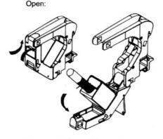
Use screwdrivers or fingers to open the poles at the top of the module.
