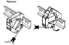
Insert a screwdriver into the opening at the bottom of the module and use it as a lever to pull out the module.
