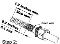
Strip off cable jacket for at least 1.2 Inches and retain a 0.2 Inches foil from cable end.
