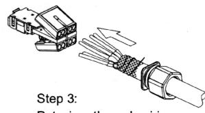
Put wires through wiring management in accordance with wiring color code.
