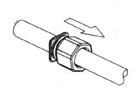
Step 1: Put cable through the Nut. (OD:6~8mm;23~26AWG)
