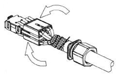
Step 4: Press wiring management to terminate wires.
