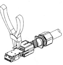
Step 6: Assemble the wiring management("UP" on the top surface) into the groove of base housing, and locate the nut
