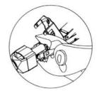
6 Close connection module cover, make sure the drain wire is in proper contact with grounding clip on connection module. Pull back strain relief boot to cover the connection module, fasten supplied cable tie to secure grounding contact.
