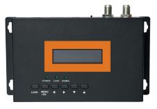
**1. LOCK:** (DOUBLE USE BUTTON): 1. locks the use of the buttons. "LOCK" led lights up when pressed 1 time for locking. To release lock state, press again. 2.also functions as "Delete" (Space) button while editing menu "Name".
